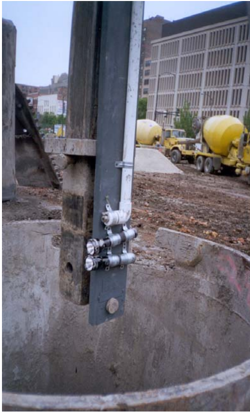
“SeeSnake” fiberoptic viewer attached to Kelly bar, with lighting
