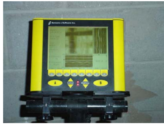
The CONQUEST Impulse Radar monitor screen shows the location and depth of embedded objects
