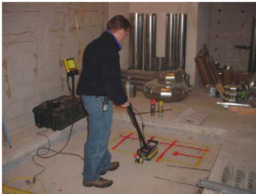
GME engineer scans the concrete slab for rebar locations
